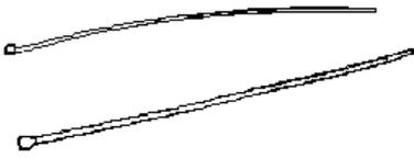
**Step 2.**Loop each cable tie through the mounting bracket hole at the top and bottom. Wrap them round the pole and tighten the cable ties to secure the unit to the pole.
